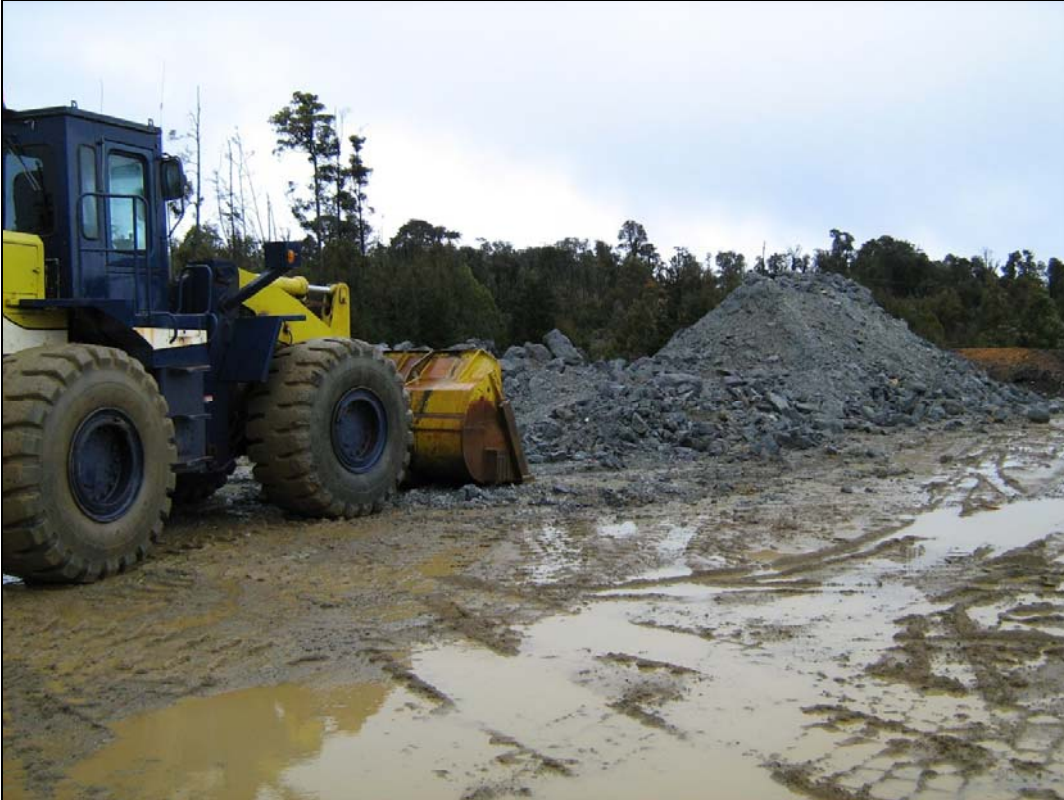
Figure 1: Front end loader picking up ore from the Medium Grade stockpile
