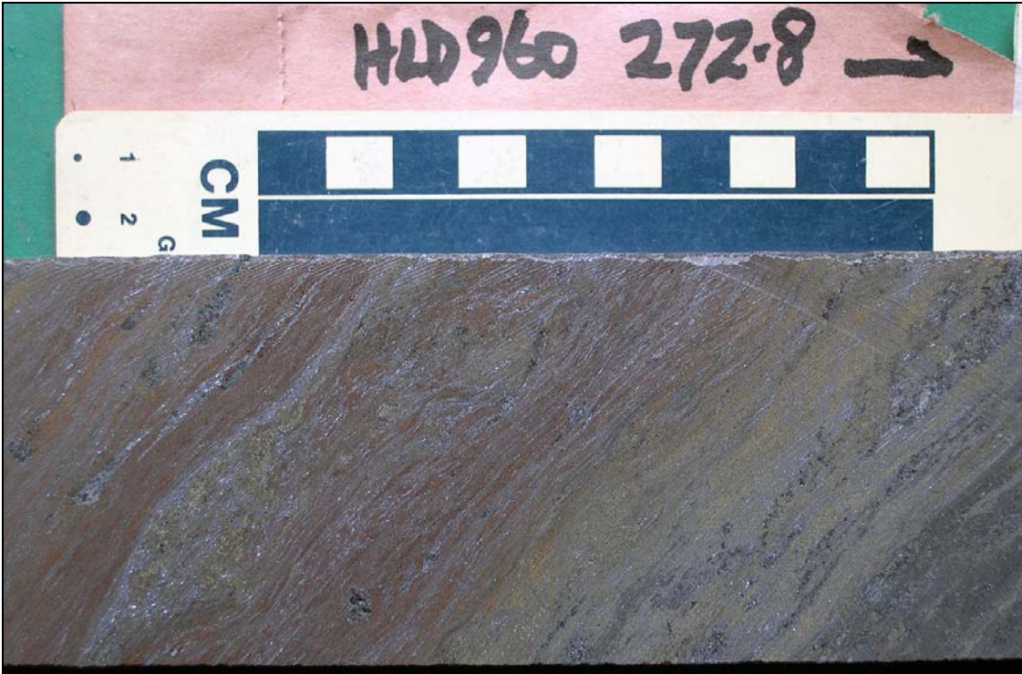
Figure 4: High grade banded base metal sulphides from the lower high-grade intercept in HLD960.
