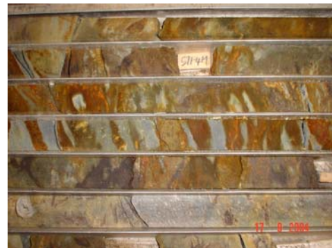
Que River drill core - stringer copper zone
